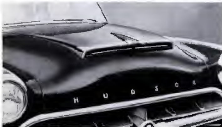
HUDSON lowered its hood and added a broad air scoop that admits air into top of engine compartment
